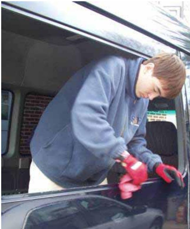
Remove the glue and dirt from the pinch weld flange.
