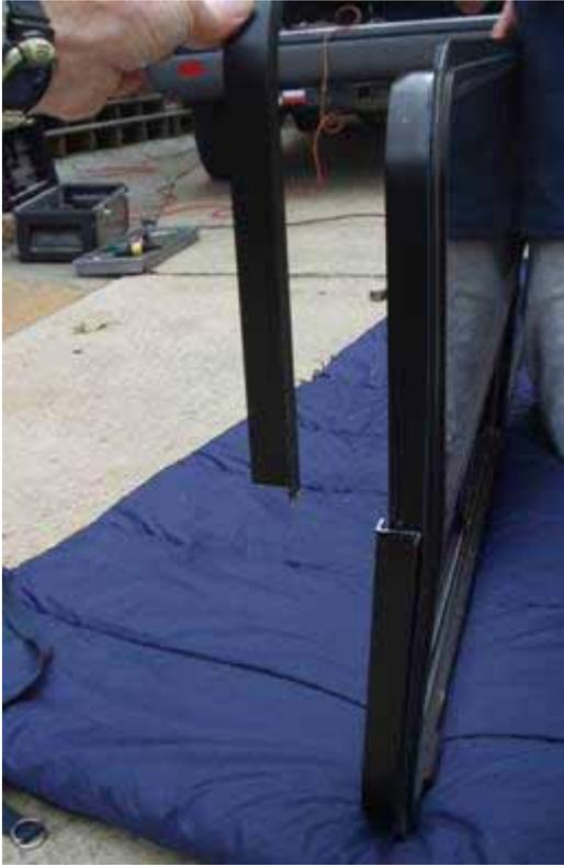
A step back: The instructions provided by Peninsula show a diagram on how to apply the compression frame. However, the diagram is incorrect, as it shows a “S”- frame with the outer flange extending away from the window to accommodate a thick wall. The “S” flange for the pinch-weld window must go under the window to reach the wall of the van.
