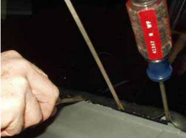
Start prying up the window gasket from a lower corner. Flat screw drivers work fine. The gasket was still quite flexible at 50-degrees without the need of heat.
