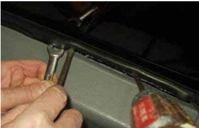
Start pushing the lip of the gasket over the pinch weld.
