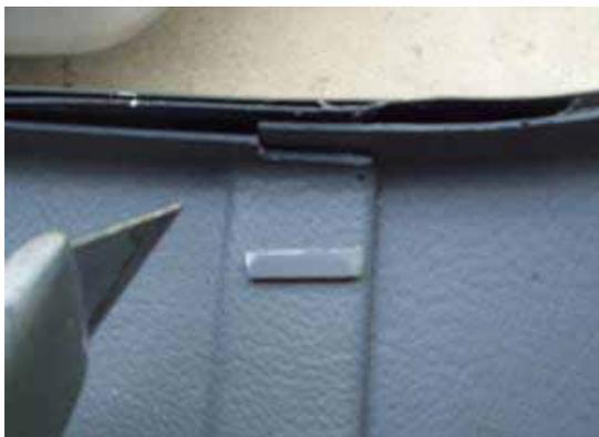
The new window's compression strip goes over the plastic. There is no gasket on the inside to fill in any gaps. Therefore, reduce the bumps by trimming the four places around the window that the plastic overlaps.
