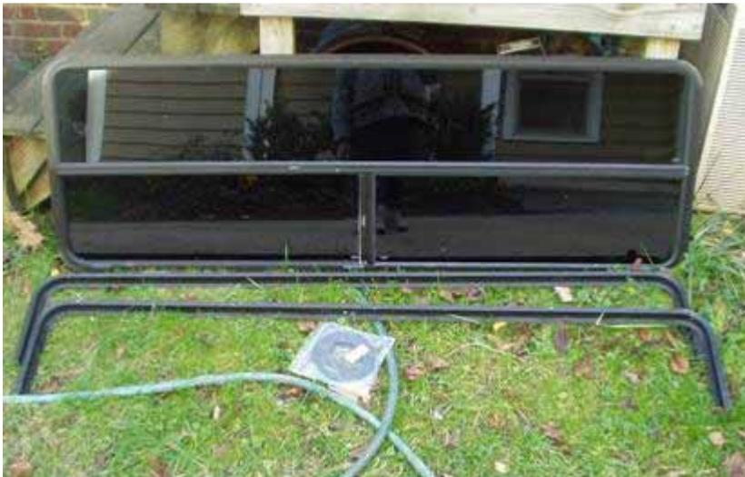
The window comes with two compression frames, double-backed foam, stainless steel sheet metal screws, (allegedly) two plastic shims and somewhat useful set of installation instructions.
