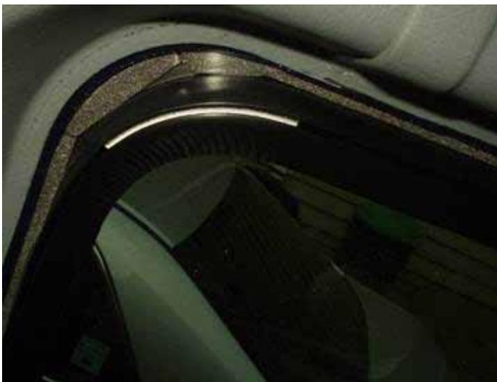
This is how the corners look with the window properly shimmed. The exterior aluminum frame covers the skin of the van. There are no gaps between the window and the skin of the van.
