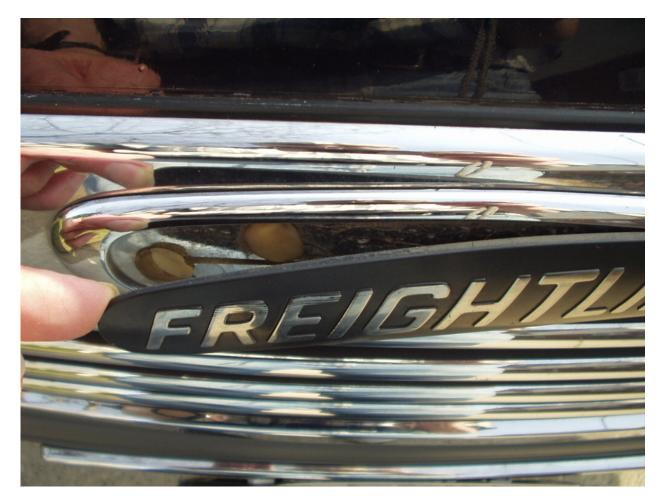
Once the emblem is off, note that the glue dots are <u>always</u> well attached to the chromeplastic base. Do not take these dots off, as they provide the proper spacing between the base and the face of the emblem. Clean these dots with a non-grease cleaner.
